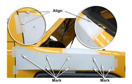
**4** Drill a pilot hole for each marked hole position.
