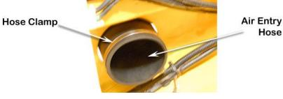
Install the modified engine air intake pre-cleaner into the air entry hose (Item 10). Fasten the engine air intake pre-cleaner using the stock fasteners.
