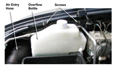
Route the overflow extension hose to meet with the standard overflow hose. Trim the standard overflow hose to the required length and join the two hoses together with the plastic adaptor (Item 21).
