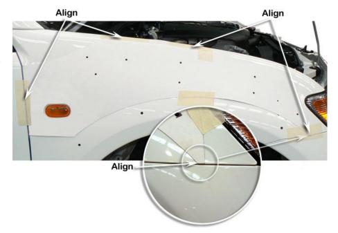
5 Drill a pilot hole for each marked hole position.
